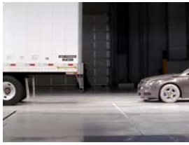
2007 Hyundai Attachments failed Severe underride with dummies' heads contacting hood/trailer
