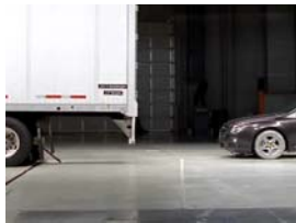
2011 Wabash No attachment failure but outboard end bent forward No underride
