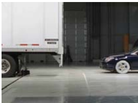
2011 Wabash Outboard end bent forward Severe underride with dummy's head contacting trailer
