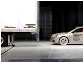
2007 Vanguard Attachments failed Severe underride with dummy's head contacting trailer
